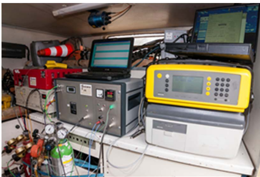
Figure 2: MIP-system next to GC/MS (HAPSITE)
