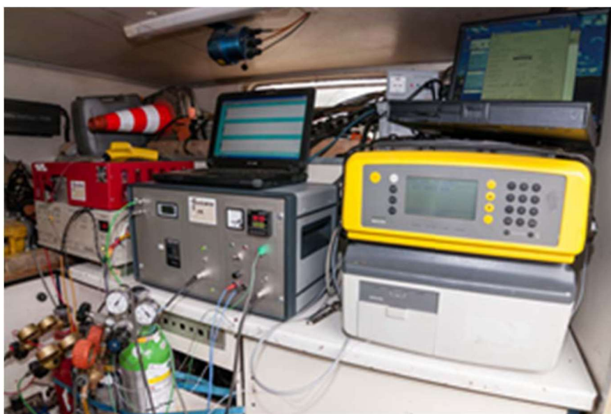
Figure 2: MIP-system next to GC/MS (HAPSITE)
